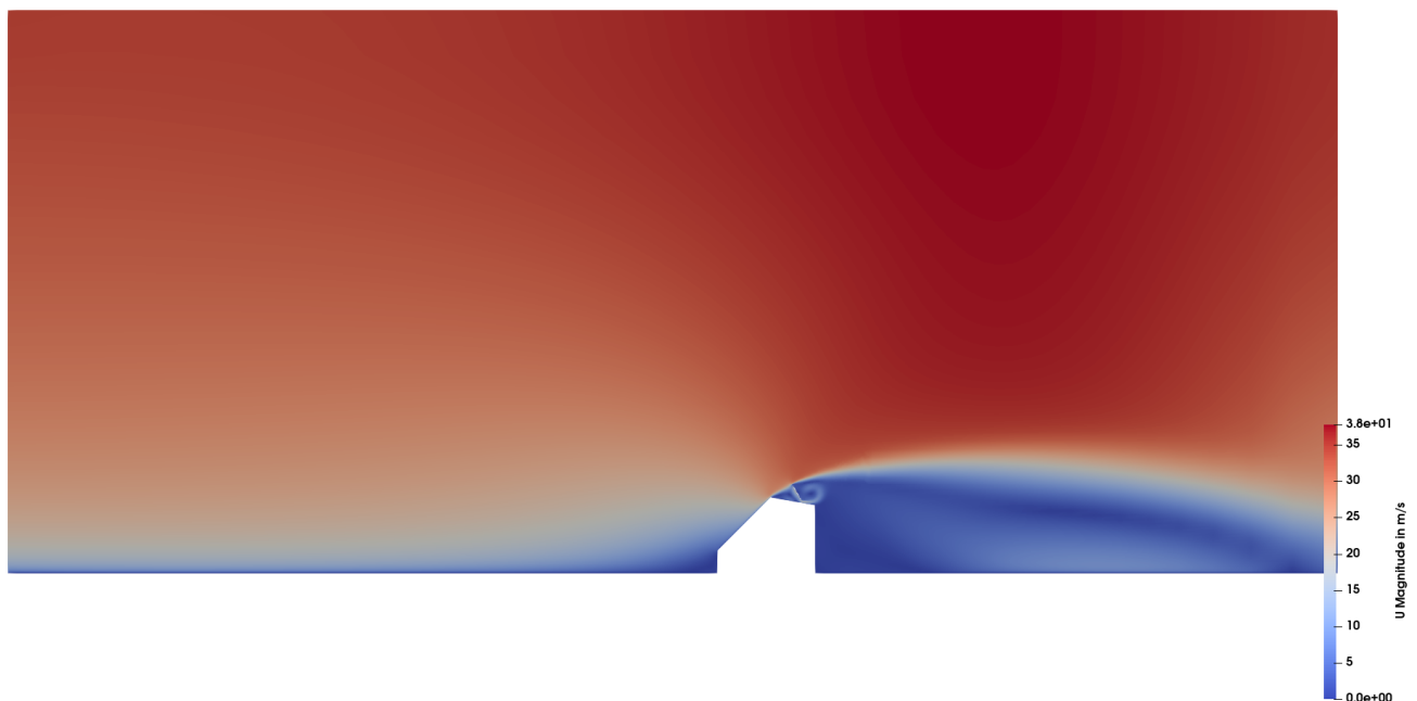
Fig. 4: Figure of the model domain containing a distribution of wind speed U in m/s around the solar panel. The wind flow direction is from left to right. Note that the panel might appear very small due to the large domain size.
