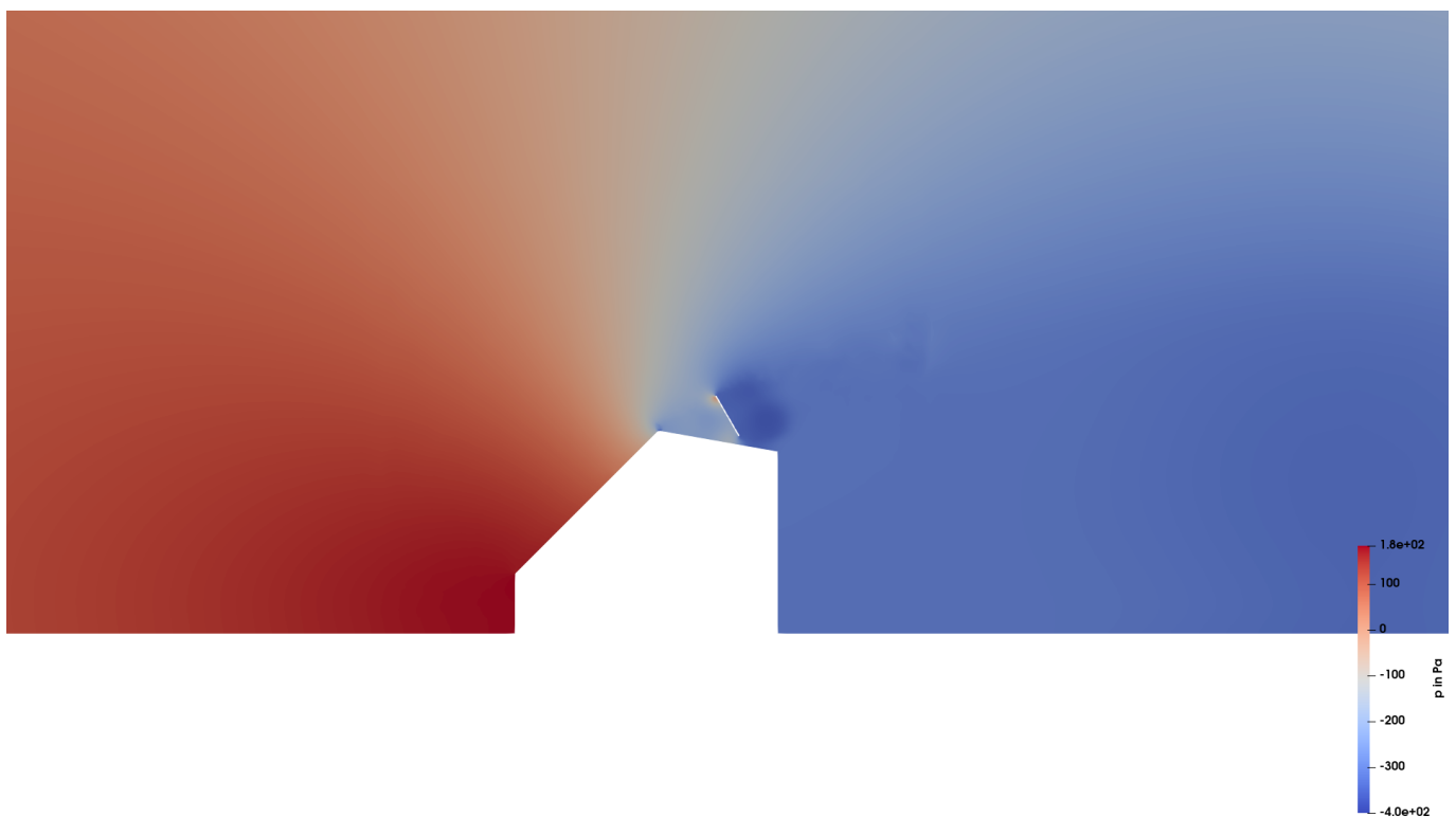
Fig. 6: Closeup-figure of the relative air pressure p in Pa around the solar panel.
